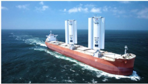
The WindWings sails by BAR Technologies look and work a lot like airplane wings. (BAR Technologies)
