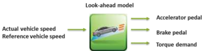
FIGURE 5-15 - AUTONOMIE DRIVER MODEL
