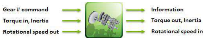
FIGURE 5-6 - AUTOMATIC GEARBOX MODEL INPUT/OUTPUT
