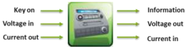
FIGURE 5-14 - AUTONOMIE ELECTRICAL ACCESSORIES MODEL
