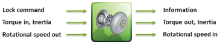
FIGURE 5-9 - AUTONOMIE TORQUE CONVERTER MODEL INPUT/OUTPUT
