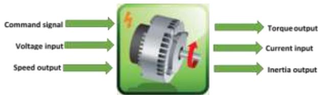
FIGURE 5-12 - AUTONOMIE ELECTRIC MACHINE MODEL INPUT/OUTPUT
