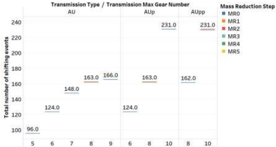
FIGURE 5-16 - TOTAL NUMBER OF SHIFTING EVENTS FOR AUTOMATIC TRANSMISSIONS
