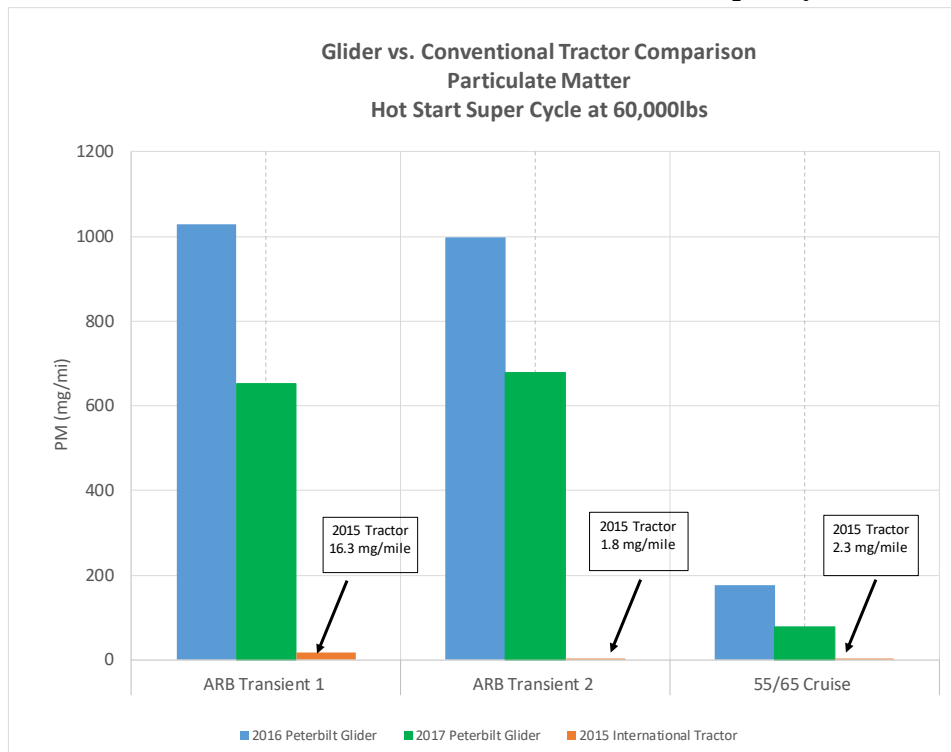
Figure 13: PM Emissions Comparison of 2015 MY Day Cab to the 2016 MY Peterbilt 389 Glider #1 and 2017 MY Peterbilt 579 Glider #2 over the Super Cycle
